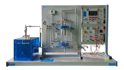
\*The picture shown are heat exchanger base unit with optional item film and dropwise condensation unit
